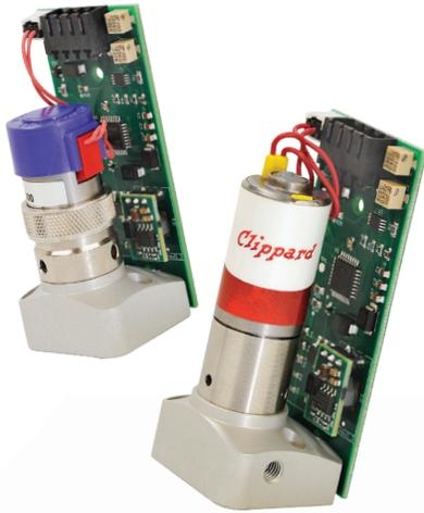
Clippard's Cordis CP1 Pressure Controller utilizes Clippard's proven EVP and DVP proportional valves to allow for steady, accurate, repeatable downstream pressure control as demand or process changes. The result is incredibly precise, linear pressure control within a closed-loop system that provides ultra-high resolution and repeatability.
